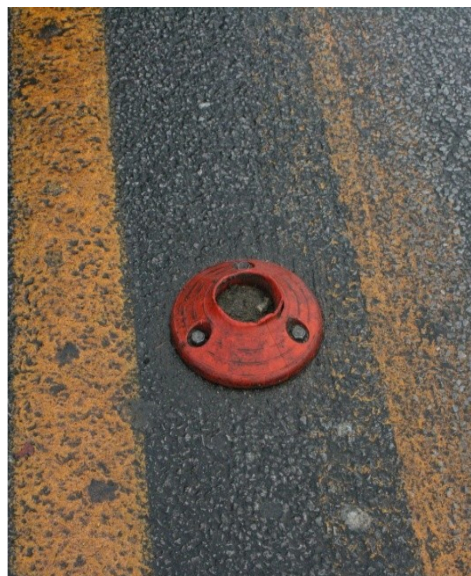
Damage due to concentration of tensile strength at the cross section area
