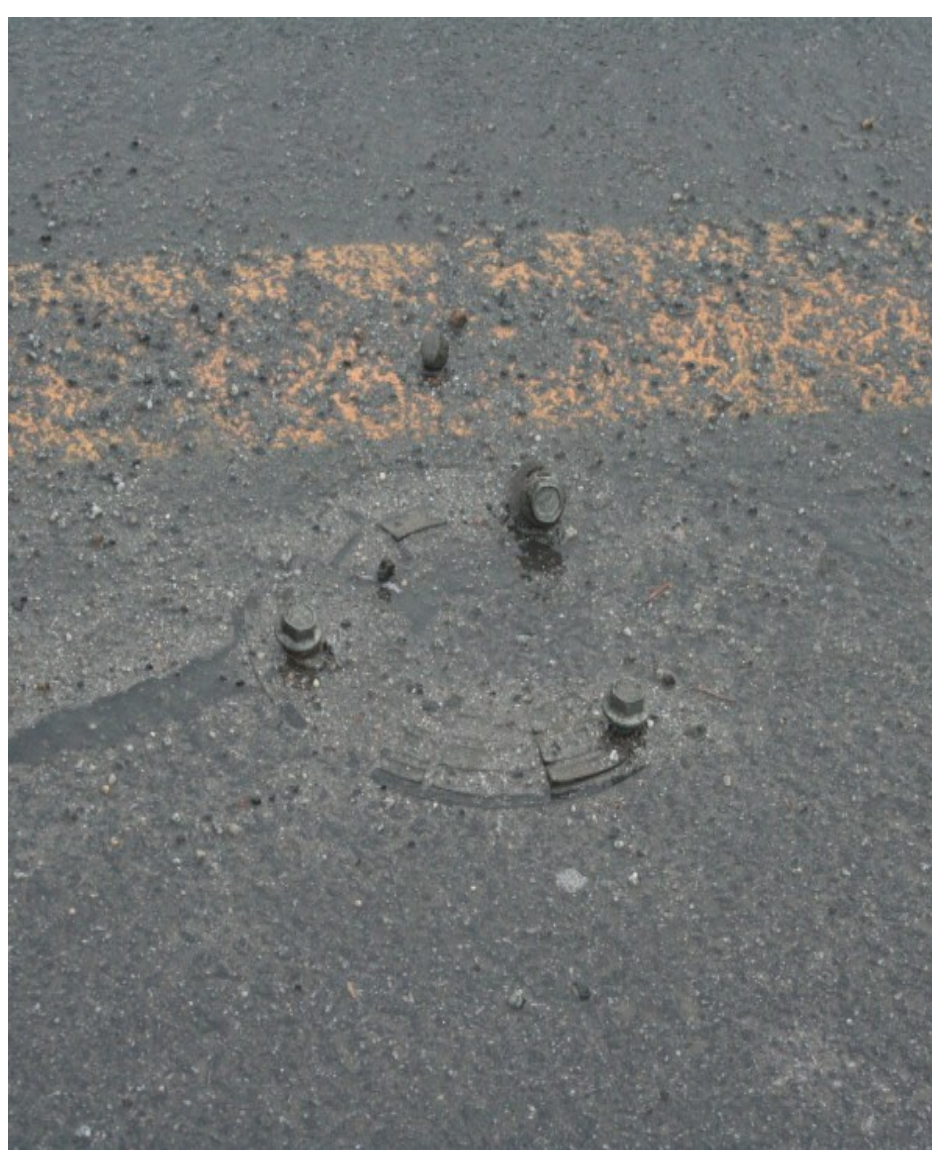
Loss due to lack of tensile strength of the lower fixing plate
